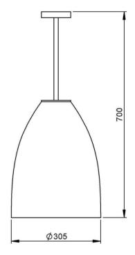
Dimensions in mm and approximate Height can vary based on project requirements
